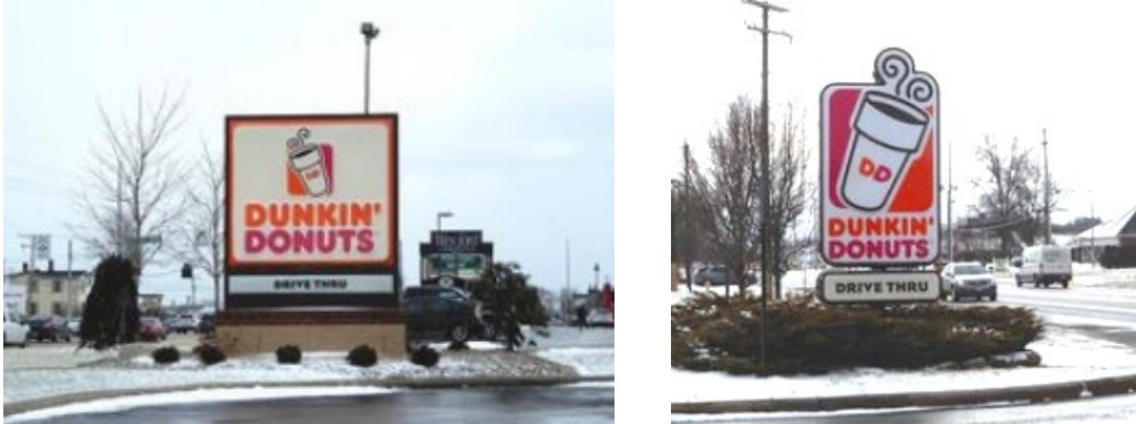
Figure 12.11-A: The sign on the left is a freestanding monument sign on a solid base. The sign on the right is a cabinet sign mounted on a pole, screened by landscaping. Both types are permitted.
