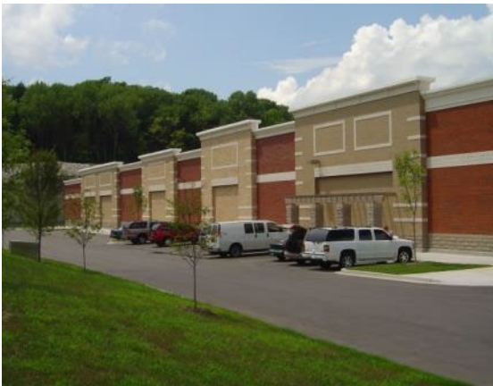
Figure 9.04-A: This figure shows two methods of using architectural features to create wall surface relief on wall elevations that are not the primary elevation.
